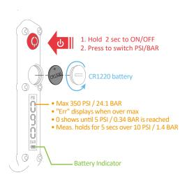
• To reset the gauge: TURN THE PUMP ON FIRST, then press and hold the power button for 10 seconds. The gauge will turn off and on during this process, do not let go of the button until the gauge turns on again.
